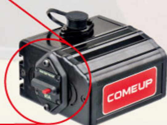
► The over-load protector built-in the control box designs to prevent overheating of the winch
