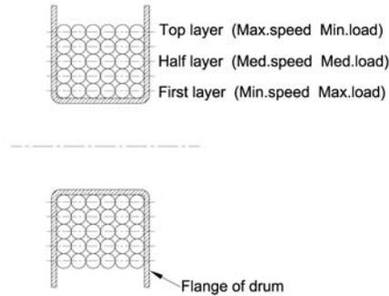
According to EN 14492-1 Section 5.7.2, the flanged drum end plates shall protrude beyond the rope wound on the drum at the top layer by at least 1.5 x the nominal rope diameter.
